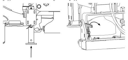
STEP 2: If using the post pulling chain as a plumb bob and/or depth gauge, attach the post pulling chain to the post pulling bracket.
