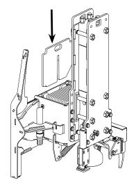
STEP 3: Reinstall the cover plate and secure with the four (4) bolts and lock washers.
