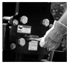
STEP 4: Have the helper remove the large retention pin from the right side of the Hornet. Use the smaller retention pin to push the larger retention pin out until it can be grasped and pulled by hand. If the driving tool is properly supported, the large retention pin should slide out with ease.
