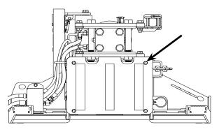
STEP 2: Starting at the front of the weight box, insert ballast plates as shown.
