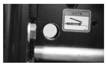
STEP 10: Have the helper reinstall the large retention pin with the groove oriented to the right of the Hornet. (When the large retention pin is properly installed, the ends of the pin will be flush with the power cell on both sides.)
