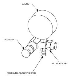
STEP 5: **SLOWLY** open the pressure adjusting knob. The compressed nitrogen will now be released to the atmosphere. Once the pressure gauge reads 0 with the plunger pressed in, the nitrogen chamber is empty.
