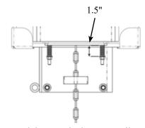
Tighten tensioning nuts until springs are adequately preloaded
