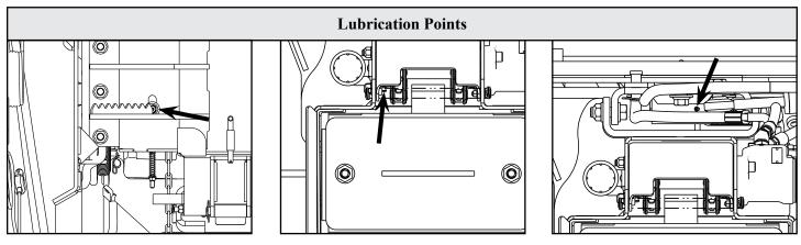
Chain Sprocket Shaft - 1 Zerk
