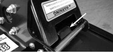
STEP 5: Slowly lower the Hammer onto a flat, level surface, or use blocking to securely support the Hammer.
