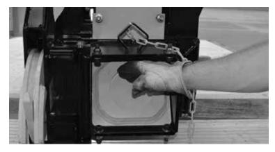
STEP 9: Using the vehicle, slowly tilt the Hammer to the upright position. Once the weight begins to slide down the Hammer case, momentarily stop tilting the Hammer so the weight can slowly slide to the bottom of the case.
