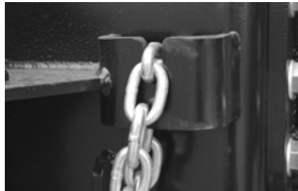
Skid-steer mounted Hornet post pulling bracket
