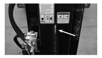
STEP 2: Using the vehicle, lower the Hammer onto the top of a previously driven post, ensuring the post is inside the lower portion of the Hammer. Continue lowering the Hammer, allowing the top of the post to make contact with the strike plate in an attempt to clear the jam. It might be necessary to raise and lower the Hammer onto the top of the post several times to clear the jam.
