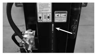
STEP 2: Ensure the retention pin is in place. The retention pin prevents the hammer weight from sliding out of the Hammer.
