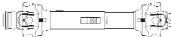
End Yokes Properly Aligned
