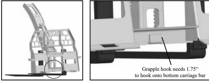
**NOTE** The 170500 Multi-Purpose Grapple fits most other pallet fork frames. See the diagram below for proper frame design.
