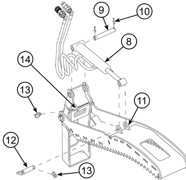
STEP 6: Route hydraulic hoses out of the way, and connect them to the vehicle's auxiliary hydraulics. Test the vehicle to make sure you have enough hose length to perform the full range of the loader arms' operating heights.
